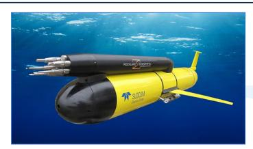
Autonomous underwater vehicle, operating along vertical sections to monitor the water column up to 1000 m depth. It provides vertical profiles of hydrological properties and turbulence through continuous cycles of immersion-emersion. The system was acquired by CNR in 2014 as part of the project EUROFLEEETS.
