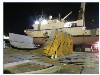
RV "Minerva UNO" with the RV "Urania" new 6 meters section
