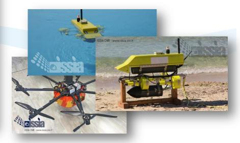
"Shark is the little autonomous semi-submersible robot that measures the environmental parameters and perform the water sampling at the air-sea-ice interface. It is fitted with a compass and GPS, automatic control systems, and a radio to transmit images and telemetric values as well as receiving instructions. The drone is technology-intensive. It navigates with support from a flying drone with eight propellers, who can photograph and videotape the surface of the glaciers"
