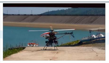
Length: 2.170m Width: 0.70m Heigth: 0.980m MR Diameter: 2 x 2.80m Dry Weight: 37 Kg Fuel capacity standard: 6L Max Fuel capacity: 20L (optional) Endurance 6 L (20 L) Fuel: 50 (200) min Payload 6 (20) L Fuel: 26 (18) Kg Max Airspeed: 80 Km/h Engine: 19.5 Hp Fuel Type: gasoline Generator: 200W OAT: "-10° C / +35° C" Max Crosswind: 24 Km/h
