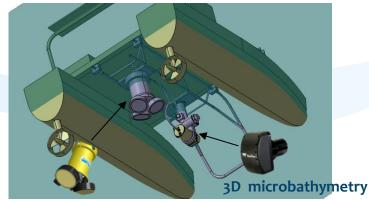
Length: 2.00m Width: 1.50m Draugth Heigth (with roll bar): 0.40m @120 Kg Heigth: 1.20m Hull: 35Kg Thrusters: 10 Kg Box control: 10 Kg Battery box: 30 Kg Max payload (including box payload): 35 Kg Power engines:  $300 \text{ W}(x_2)$ Engines push forward: 13 Kgf  $(x_2)$ Thrust engines in reverse:  $12.8 \text{ Kgf}(x_2)$ Supply voltage (min-max): 35-55 V Supply voltage (nominale): 46.8 V Capacity: 69.6 Ah Charging time: 12 hours
