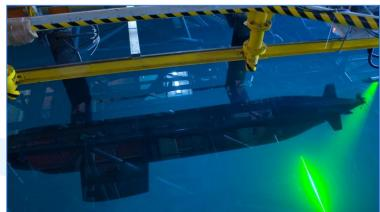
Hydrodynamic and self-propulsion test (submarine)
